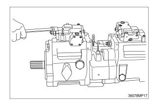
(11) Attach the PTO unit by fastening the flange socket bolt (435) to the valve block (312).
