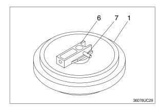
Supply engine oil to the specified level, and tighten plug.
