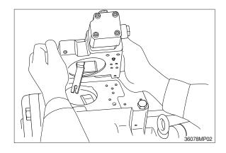
(5) Loosen hexagon screw (401) which tighten swash plate support (251), pump casing (271) and valve block (312).
