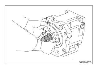
(10) Tapping lightly fitting flange section of swash plate support (251) on its pump casing side, separate swash plate support from pump casing.
