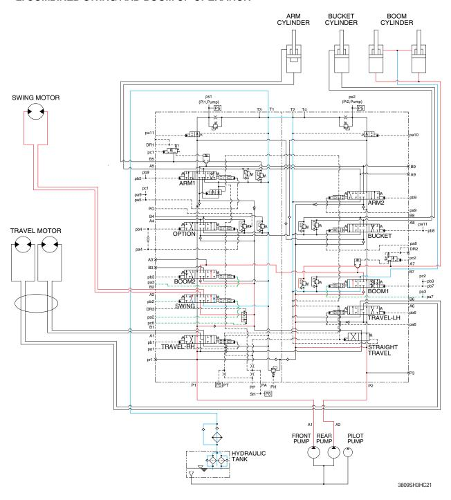
When the swing and boom up functions are operated, simultaneously the swing spool and boom spools in the main control valve are moved to the functional position by the pilot oil pressure from the remote control valve.
