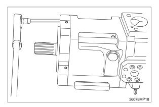
② Remove flange socket bolt (435) and remove PTO unit.
