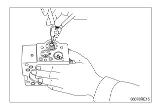
(11) Fit set spring (655) to spool hole and put compensating piston (621) and piston case (622) into compensating hole.
