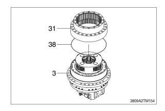
(14) Tighten hub and ring gear.
