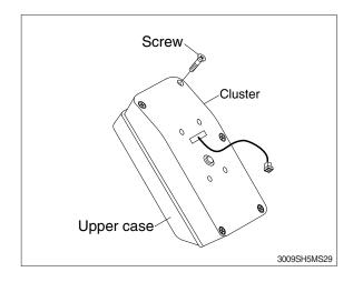
6) Install the new ROM. (Be careful of direction and assemble the cluster in the reverse order to removal).
