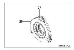
(17)After removing pin (29), remove No.3 planetary gear C (27), needle bearing (11) and plate C (20).
