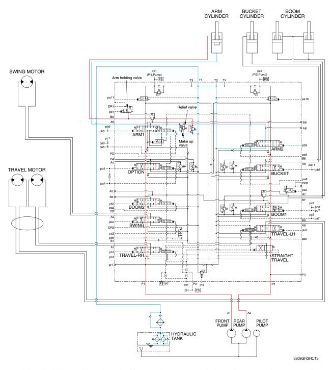
When the LH control lever is pushed forward, the arm spools in the main control valve are moved to the roll out position by the pilot oil pressure from the remote control valve.
