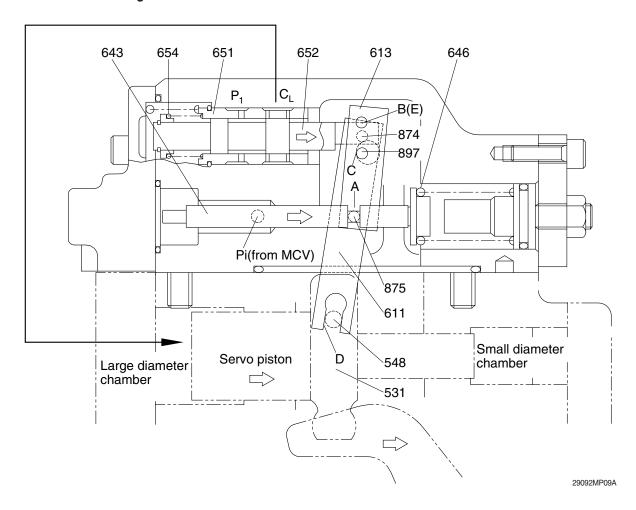
As the pilot pressure Pi rises, the pilot piston (643) moves to the right to a position where the force of the pilot spring (646) balances with the hydraulic force.
