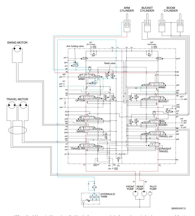
When the LH control lever is pulled back, the arm spools in the main control valve are moved the to roll in position by the pilot oil pressure from the remote control valve.
