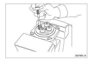
(5) Assemble O-ring (15) onto plug (14).
