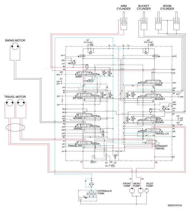
When the arm and travel functions are operated, simultaneously the arm spools and travel spools in the main control valve are moved to the functional position by the pilot oil pressure from the remote control valve and the straight travel spool is pushed to the right by the oil pressure from pilot pump.
