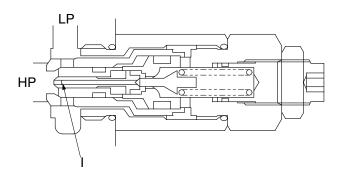
(4) The oil flow from the high pressure passage (HP) to the poppet (D) behind is only around poppet and orifice (F); then the high pressure passage (HP) is higher than the poppet (D) behind pressure. Thus the poppet (D) is pushed open and the oil directly flows into low pressure passage(LP).
