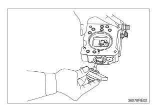
(5) After removing cover (C, 629) subassembly, take out outer spring (625), inner spring (626) and spring seat (C, 624) from compensating section.
