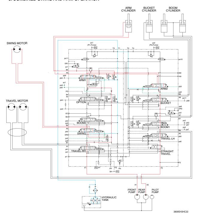
When the swing and arm functions are operated, simultaneously the swing spool and arm spools in the main control valve are moved to the functional position by the pilot oil pressure from the remote control valve.
