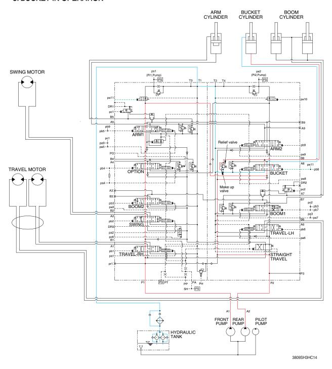
When the RH control lever is pulled left, the bucket spool in the main control valve is moved to the roll in position by the pilot oil pressure from the remote control valve.
