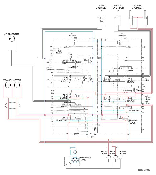
When the boom and travel functions are operated, simultaneously the boom spools and travel spools in the main control valve are moved to the functional position by the pilot oil pressure from the remote control valve and the straight travel spool is pushed to the right by the oil pressure from pilot pump.
