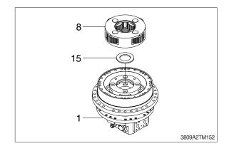
(12) Press-fit ring (39, 40) to the No.1 carrier A (8) assy.
