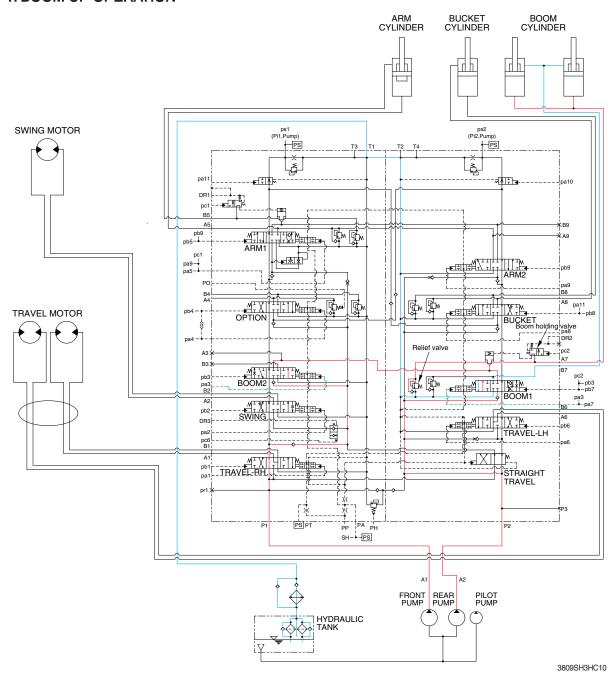
When the RH control lever is pulled back, the boom spools in the main control valve are moved to the up position by the pilot oil pressure from the remote control valve.
