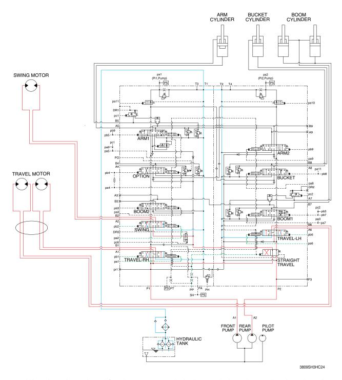
When the swing and travel functions are operated, simultaneously the swing spool and travel spools in the main control valve are moved to the functional position by the pilot oil pressure from the remote control valve and straight travel spool is pushed to the right by the pilot oil pressure from the pilot pump.
