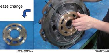
(6) Remove brake springs (25) and take the brake piston out by screwing a M16 screw into the brake piston.
